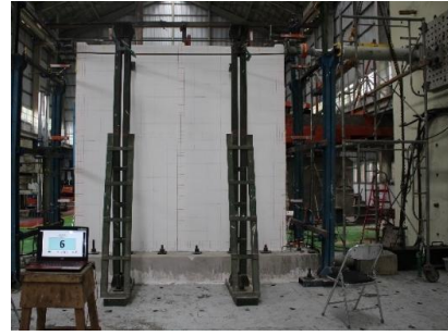
Figure 18 RUCAST 2D Wall Cyclic Test Setup.
